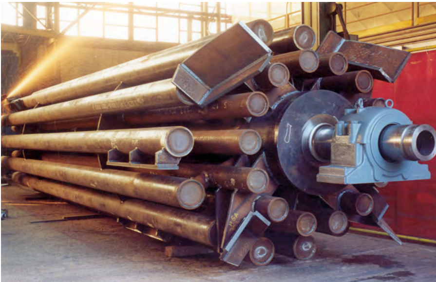
PHOTO OF ROTATING TUBE BUNDLE BUILT TO ASME SPECIFICATIONS TO 150 PSI
